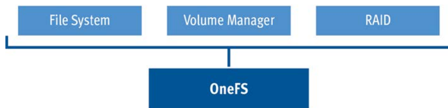
Figure 3. OneFS eliminates need for separate file system components
